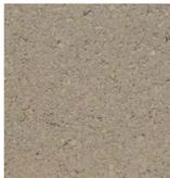
(1) Block strength of 7.3 N/mm<sup>2</sup> or greater. (2) Block strength of 7.3 N/mm<sup>2</sup> or greater. (3) Blocks are not weatherproof nor waterproof and are not suitable for unfinished external applications. External leaves must be protected e.g. render, cladding.
