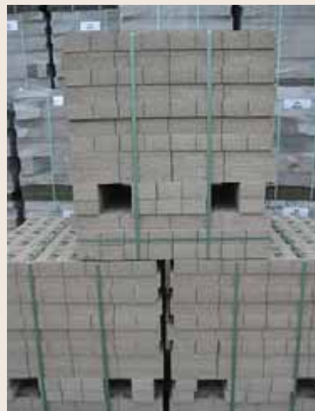
Void packed and banded
